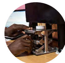
Step 5 Run through a mid- infrared spectrometer to determine soil make up
